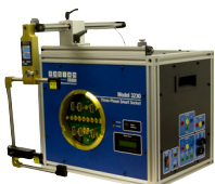
(AE0016XX) Model 3230 M3230 3-Phase Shop Stand Adapter for RW-3X, Integrated Smart Socket, USB Interface ---- This allows you to utilize the RW-3X's features while on site in the van, as well as back at the shop. See the following page for additional information.
